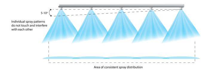
Another method to compensate for the uneven fluid distribution in a spray is to over spray a product. If a single nozzle is responsible for coating a product as it passes under it then the spray pattern can be deliberately angled so that it is wider than the target. In this way the product passes under only the middle, and hence more even, part of the spray. The obvious disadvantage of this is product waste.
