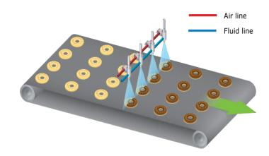
**Stop start spray line** – the target is moved on a conveyor or in spray tunnel to a spraying point where it is stopped and sprayed for the desired period before being moved on.
